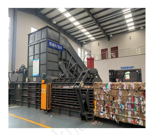
Specially used for recycling waste paper, cartons/cardboards trims/scraps etc. which are popular in packaging/corrugation industrial, paper/ printing plants etc.
