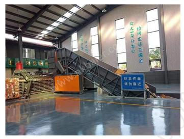
NickBaler Hydraulic fully automatic baler specialized in recycling and compressing the loose materials like plastic films ,PET bottles, plastic pallets ,waste paper ,grass ,fiber ,used clothes ,cartons ,cardboards trims ,scrap ,etc . The Nick baler Horizontal automatic Baler is ideal for warehouses and designed for ease of installation, operation and maintenance.
