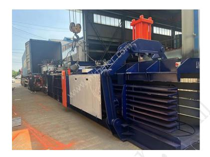
NKW180Q Cardboard Box Paper Baling Press. hydraulic baling press is generally accomplished by hydraulics. Loose materials are compressed and conformed to a particular shape, and then wrapped to maintain the shape. These bales of material have a standardized size, can be loaded to consist of a standard weight for easier transportation and storage.
