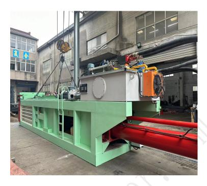
Special used in recycling and compressing the loose materials like plastic film, PET bottles, plastic pallets waste paper cartons, card boards trims/scraps. etc
